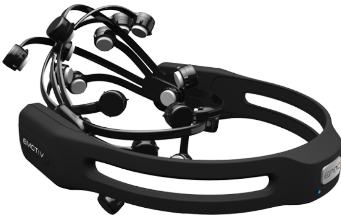
Figure 4.4: Image of the Emotiv EPOC+ Headset. Image Credit: Emotiv Inc. Digital image. Accessed April 13, 2017. Retrieved from https://www.emotiv.com/epoc/
